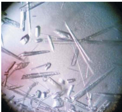
Figure 1 Crystals of untagged apo-GAPDHA grown in 100 mM HEPES pH 9.0, 17% PEG 8000. Crystals grew to 200 \times 50 \mu\text{m} .
